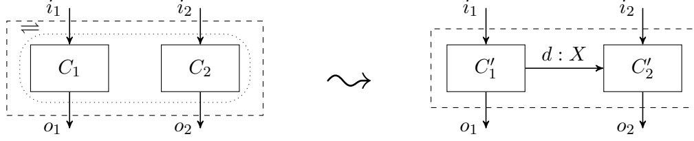
Figure 7.3: Replacing dependency (left) by an explicit channel (right).
