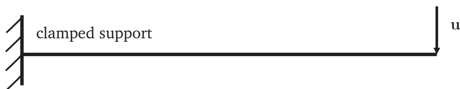
Figure 5.18: Boundary and loading conditions of the beam model. The beam is clamped at its bearing point, where the tip of the beam is displaced by 1 % of the beam length.
