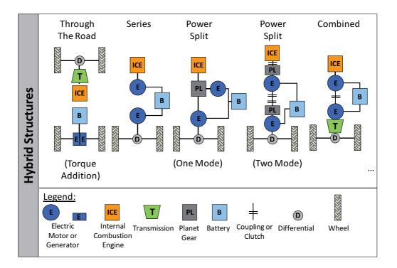
Figure 4-14 Examples of multiple HEV architecture structures
