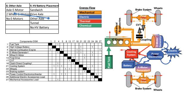
Figure 5-23 Choice selection path for a "full hybrid through the road" architecture along with schematic showing energy flows and a components-DSM depicting physical connections dependencies
