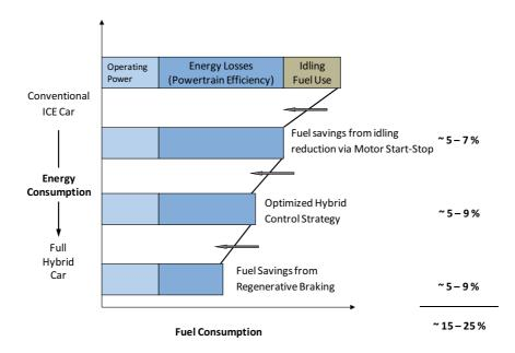
Figure 4-17 Fuel consumption saving potential for full hybrid systems [NAUNIN 1989]
