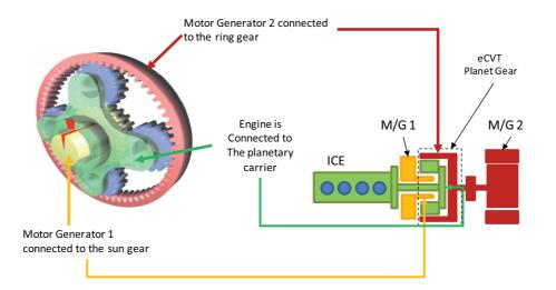
Figure 4-24 Diagram of an eCVT Planetary Gear Transmission in a One-Mode Power Split Hybrid
