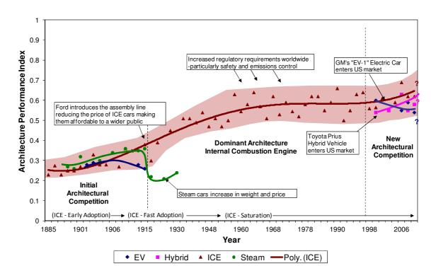
Figure 2-7 Performance of various automotive architectures from 1885-2008 [GORBEA et al. 2008]
