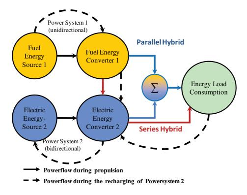
Figure 4-11 Conceptual illustration of a hybrid electric drive adapted from EHSANI et al. 2009, p.124
