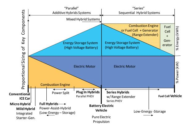
Figure 4-16 Qualitative dimensioning of key components for various car concepts and architecture structures adapted from WALLENTOWITZ et al. 1999
