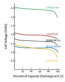
Figure 4-21 Discharge curves for various cell types at C/5 according to WOODBANK 2005
