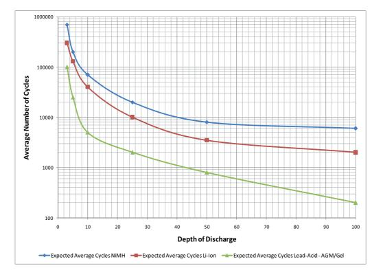
Figure 6-6 Average life of various battery technologies – Adapted from Rosenkranz in MARKEL, T. et al. 2006
