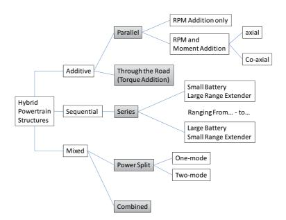
Figure 4-12 Classification tree of possible hybrid powertrain architecture structures
