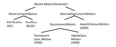
Figure 4-19 Classification of motor types
