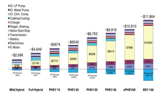
Figure 6-7 Estimated delta manufacturing costs of electrification for a passenger car 2015.
