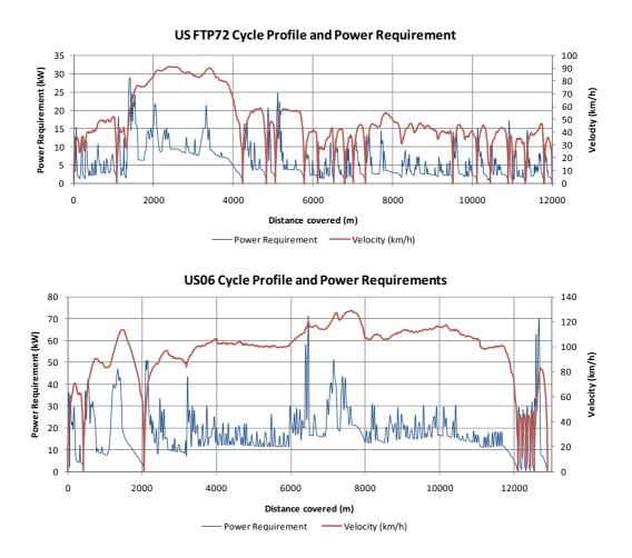
Figure 7-2 Power requirements for the electric powertrain derived from simulations using the FTP72 cycle for city driving and the US06 for highway driving – An electric motor with peak power of 70kW and sustained power of 45kW is suitable for both cycles and is selected for the subsequent analysis.
