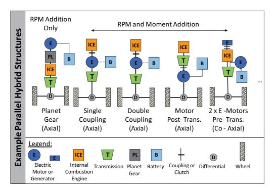
Figure 4-13 Examples of parallel hybrid vehicle architecture structures
