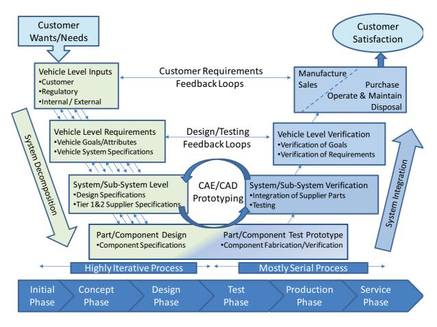
Figure 4-4 Adaptation of the Systems Engineering V-Model to Vehicle Development
