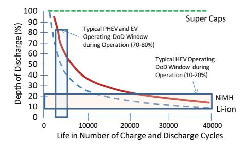
Figure 4-23 Battery Cycle Life Comparison [adapted from MARKEL, TONY 2006]
