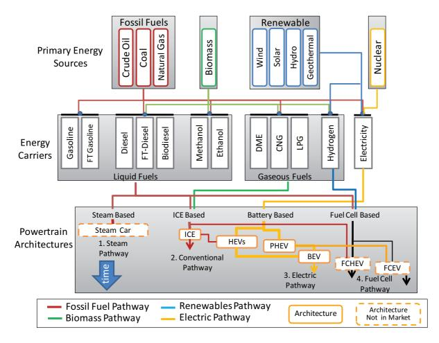
Figure 1-4 Energy to vehicle powertrain architecture pathways
