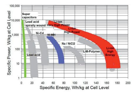
Figure 4-20 Specific Power vs. Specific Energy for various cell types from KALHAMMER et al. 2007, p.25
