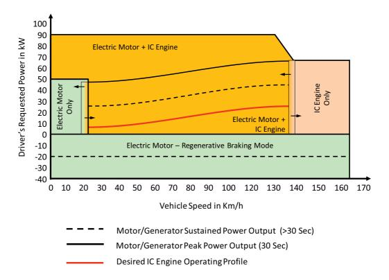
Figure 4-25 Example of a Parallel Hybrid Control Strategy [according to WALLENTOWITZ et al. 1999, p.66]
