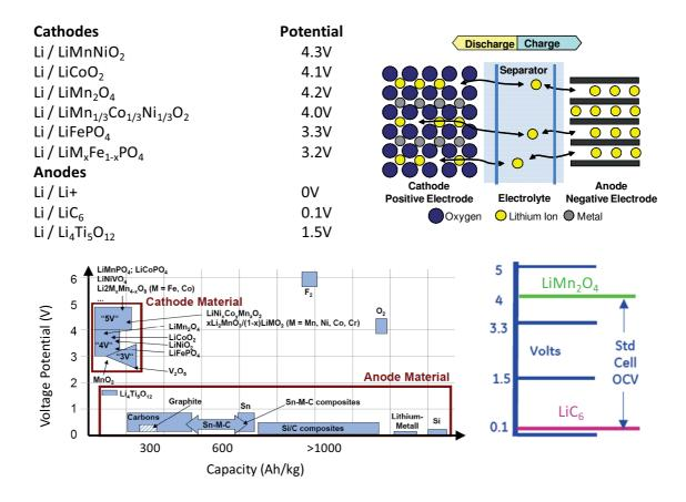
Figure 4-22 Common chemistries of Lithium Ion Battery electrodes and their open circuit voltage(top left); bottom tradeoff between voltage potential and capacity (bottom left); schematic of Lithium Ion battery structure (top right); example of standard cell open current voltage (OCV) potential (bottom right) [Adapted from SAVAGIAN 2008]
