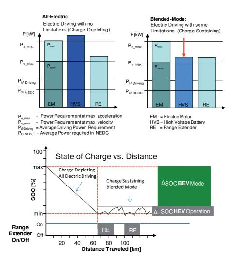
Figure 4-26 Example control strategy description for a series hybrid (graphic contributed by STEINHAUER 2009)
