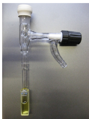
Figure 49: Modified quartz glass cell for UV-Vis investigations.
