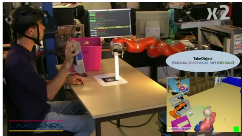
Figure 6.13: Snapshot of the film of the “Clean the Table” scenario. The physical situation, the SPARK model, and the current step of the plan can be seen.
