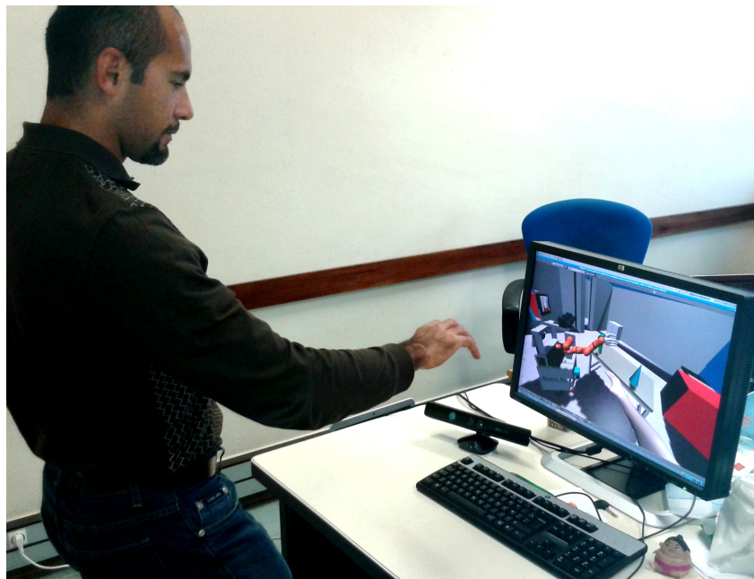
Figure 6.2: The experimental setup with the human avatar controlled from a Kinect.
