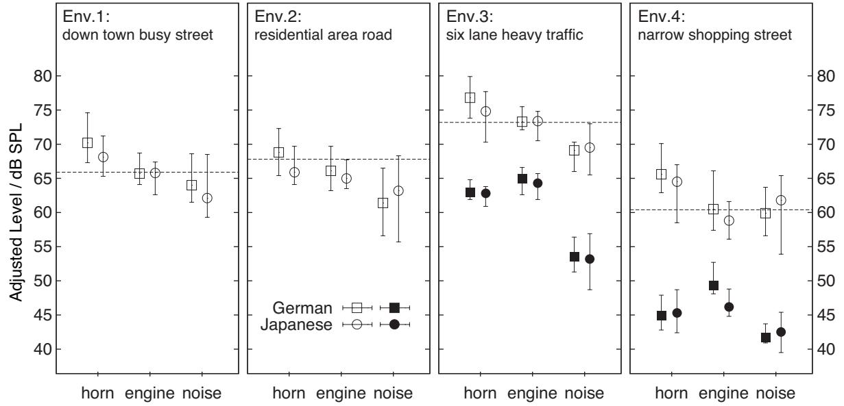
Figure 3 – Medians and interquartile ranges of the averaged adjusted levels between two trials per person. White symbols: warning sounds clearly audible. Black symbols: warning sounds just audible. Horizontal lines: level of environmental background sound.
