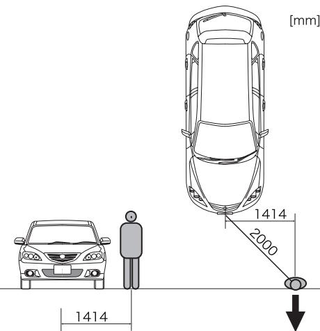
Figure 2 – Assumed relative position between the pedestrian and the vehicle providing warning sounds
