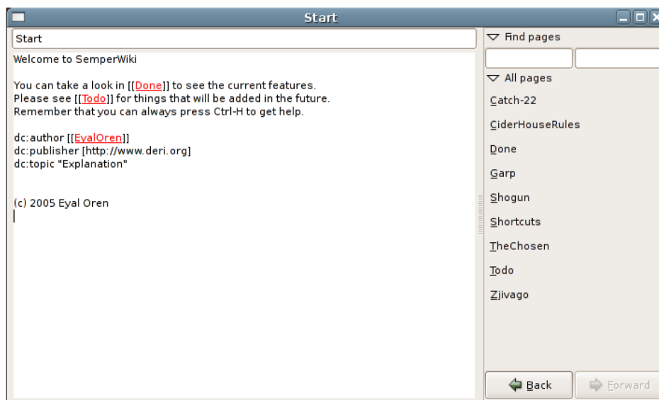
Figure 5.22.: SemperWiki editor showing keys (e.g., dc:author ) and values (e.g., "Explanation") in the wiki page content according to [Or05].
