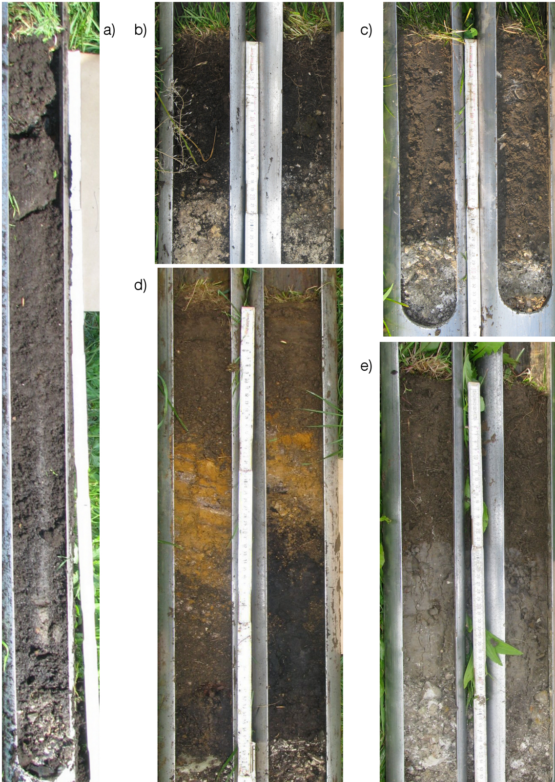
Figure A.1: Exemplary photographs of characteristic soil profiles. Two soil cores shown in one photograph have been excavated at a distance of approximately 0.5 m between each other. a) Deep peat soil, degraded near the surface due to aeration and intact in depth. b) Shallow peat soil, degraded throughout the whole profile. c) Shallow soil consisting of a single layer of humic mineral soil. d) Profile with alternating horizons of mineral soil, ochre and peat. e) Humic mineral soil with a loamy horizon of varying thickness between topsoil and gravelly substrate.
