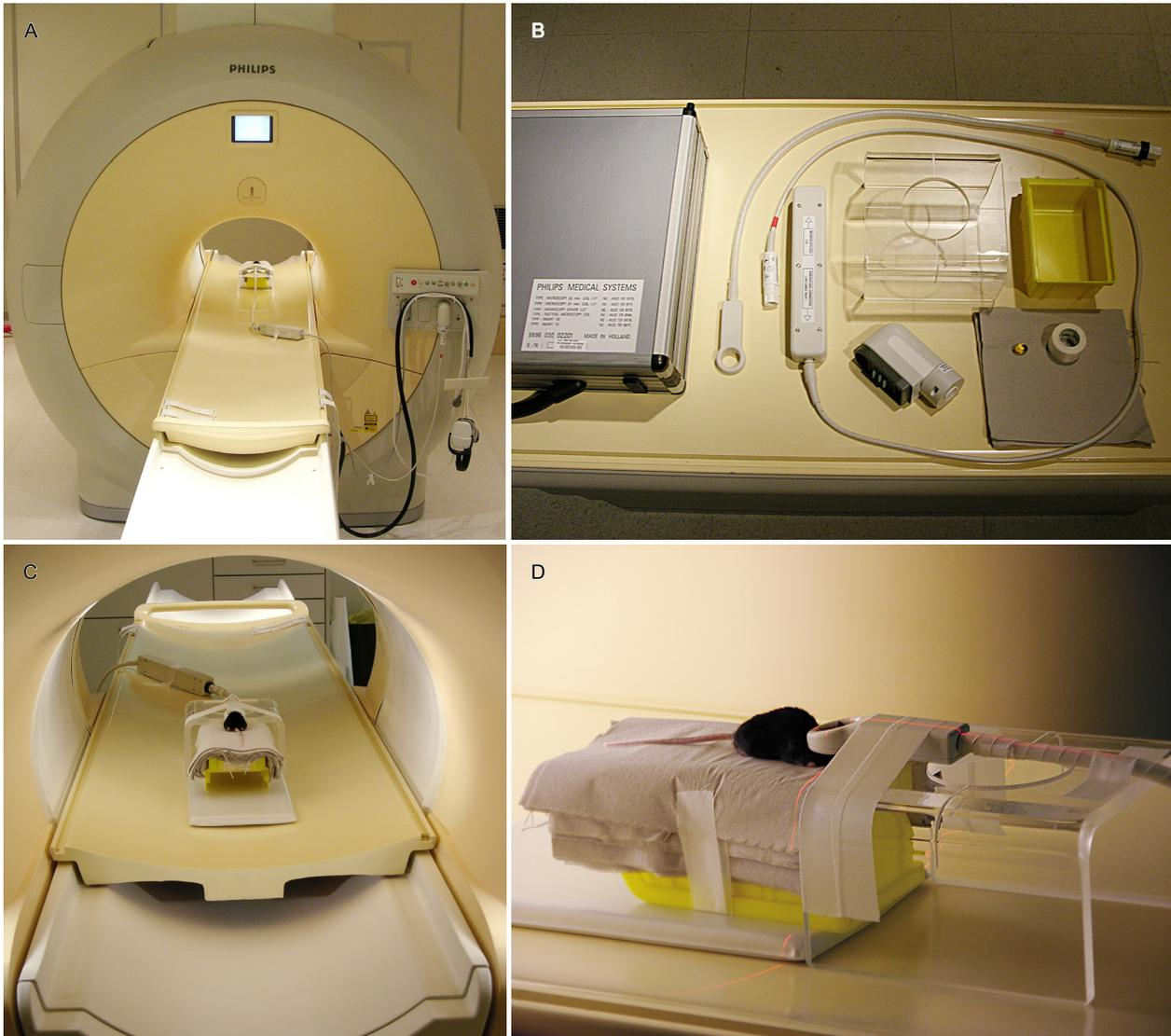
**Figure 31: Mouse brain MR imaging with Philips Achieva 1.5 T.**
