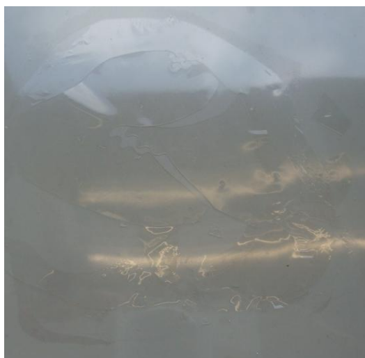
Figure 5.21. Foil (400 \mu\text{m} ) obtained from 17a-TMS with 0.1% BNT-CAT 440.
