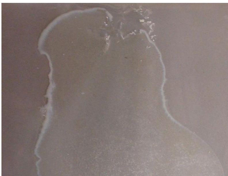
Figure 5.16. 50/50 mixture of HexMTS-AGE and glycidyl-BPA cured with DETA at ambient temperature.
