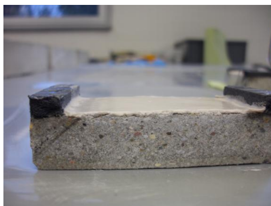
Figures 5.24. Cross section of a plate coated with 18a-TMS .
