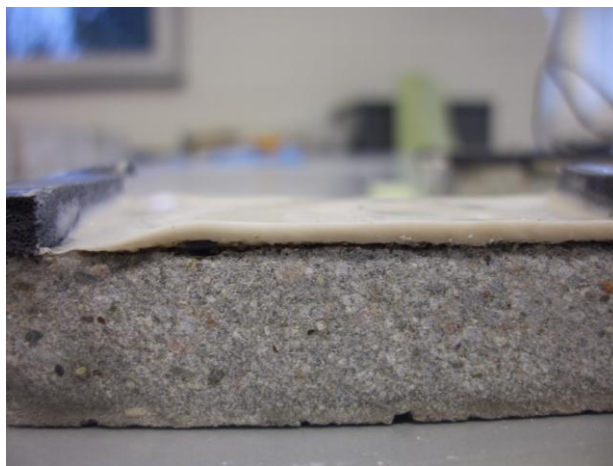
Figures 5.19. Cross section of a coated plate using 15b-NH 2 .
