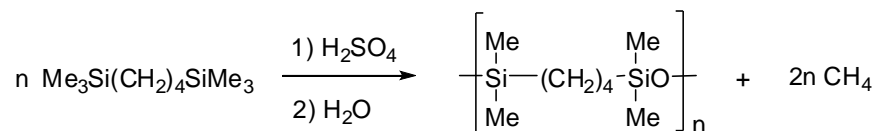
Scheme 3.1. First synthesis of hybrid silicones.
