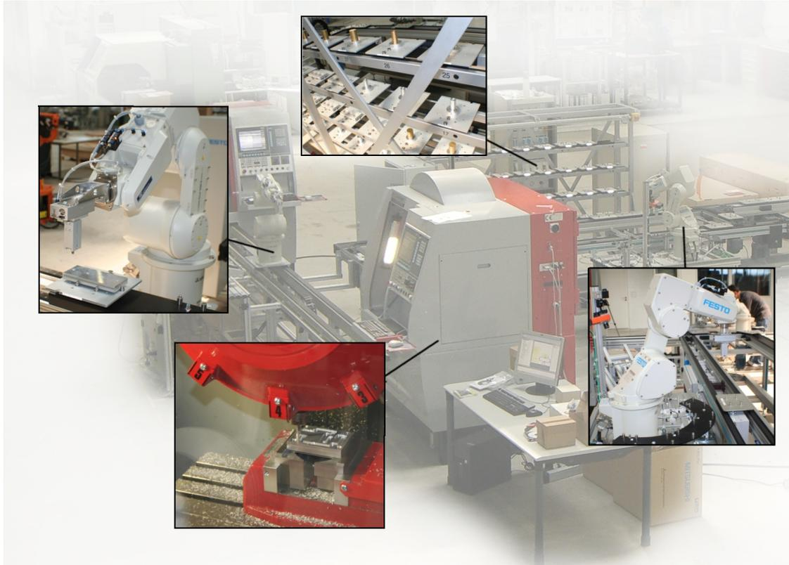
Figure 2.1.: The test-bed for the cognitive factory, an iCIM3000-based Festo flexible manufacturing system, which is part of the TUM excellence cluster Cognition for Technical Systems (CoTeSys). © Prof. Shea, TUM.
