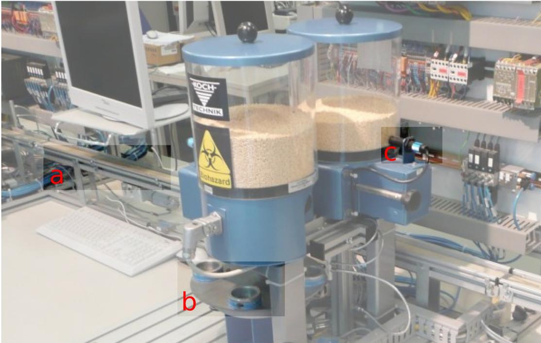
Figure 7.4.: Filling station with a) a conveyor belt that brings empty bottles, b) a swivel that moves the bottles below the nozzle of the silo and c) a photo sensor that gives a signal if the silo is empty. The bottles are placed upon the swivel by a pneumatic arm, which is not in the picture (it is behind the silos).
