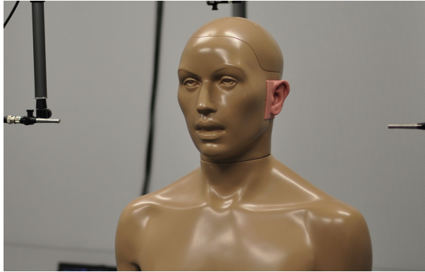
Figure 5.1: The Knowles Electronic Manikin for Acoustic Research (KEMAR) dummy head is an industry standard measurement tool. It has interchangeable ears and microphones in the ear canals.
