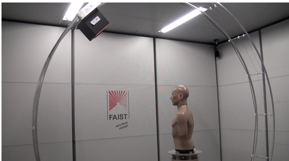
Figure 5.3: TF measurement in an anechoic chamber. The KEMAR is positioned on a turntable and a loudspeaker presenting MLS sequences is moving on the arc. The measurement is controlled by a computer and is fully automated.
