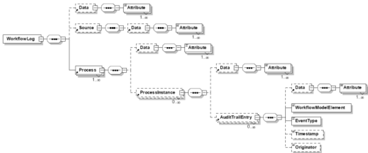
Figure 6-8 XSD Schema of the MXML format Source: Adapted from (van Dongen et al. 2005)
