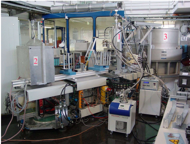
Figure 2.3: MIRA in the used set-up with cryostat (1), area detector (2) and monochromator shielding (3).
