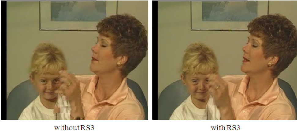
(b) Example of image quality. The video Mother&Daughter is encoded/transmitted at 500kbps/30fps without RS3 (left) and with RS3 (right). The PER is 30% and DMVE is applied for error concealment.
