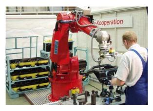
Figure 1.7: PowerMate assembly work-cell (SCHRAFT ET AL. 2005)
