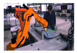
The human operator can intuitively teach a task either in the real robot cell or in a synchronized simulation model. At the Institute for Machine Tools and
