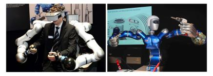
*Figure 2.4: Telepresence system for applications in space: Operator side (left) and Space-Justin as a teleoperator (right) (DLR 2011)*
