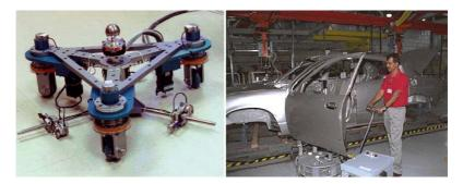
Figure 1.5: Cobot scooter (left) and assembly of car doors using cobots (right) (PESHKIN & COLGATE 1999)
