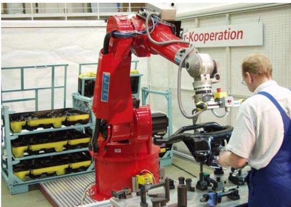
Figure 1.7: PowerMate assembly work-cell (SCHRAFT ET AL. 2005)
