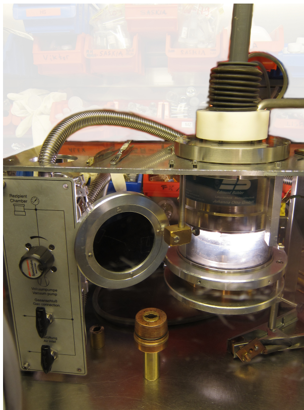
Figure 2.2 Mini Arc Melting System, MAM-1, Johanna Otto GmbH, placed in an argon filled glove box.
