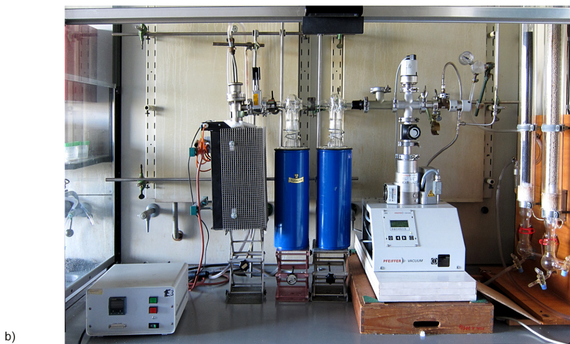
Figure 2.1 a) Schematic description of the distillation apparatus used for purification of Ca, Sr and Ba, b) photograph.
