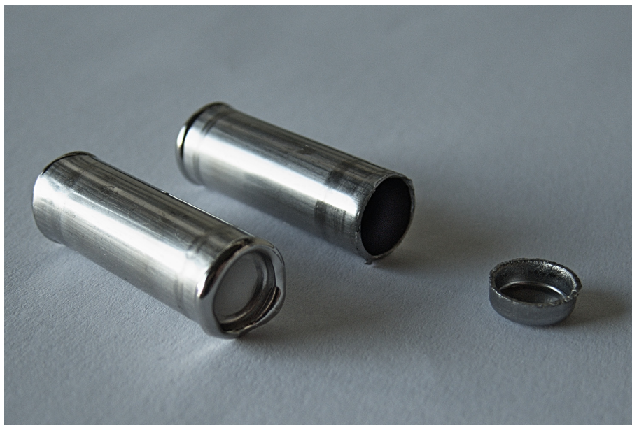
Figure 2.3 Photograph of a closed (left) and an open (right) tantalum ampoule and the corresponding lid.
