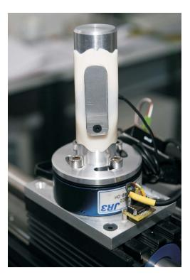
Fig. 5.2: Prototype of the grip force sensing device using one force sensor.
