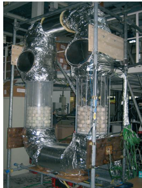
Figure 5.2: Test apparatus and prototype of PCM based HDH system
