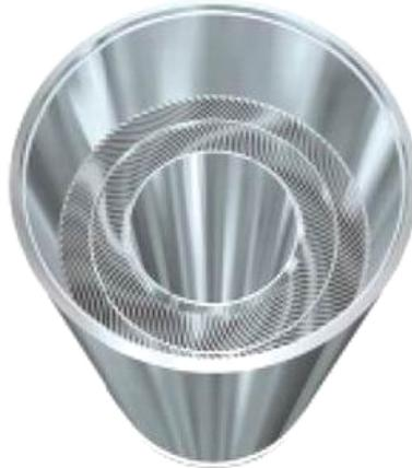
Figure 1.1: Drawing of the FRM II fuel element. The inner diameter is 118 mm, the outer diameter is 243 mm, the active height is 243 mm. The fuel element contains 113 involute shaped fuel plates, separated by cooling channels. The control rod moves inside the central hole [1,2].
