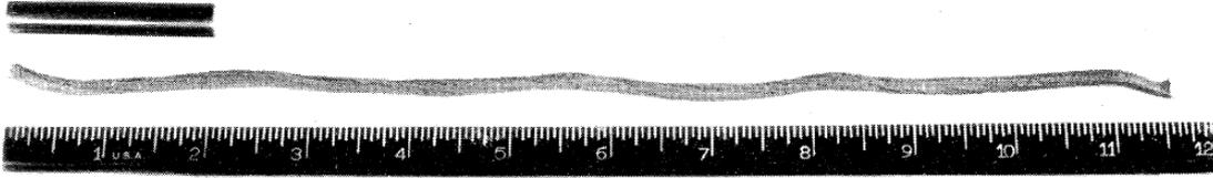
Figure 2.8: Growth of a highly textured, fine grained  $\alpha$ -uranium rod during thermal cycling. After 300 cycles from 50 °C to 550 °C the rod grew from 5 cm to 30 cm length [89]. The scalebar shown in the picture is in inch.
