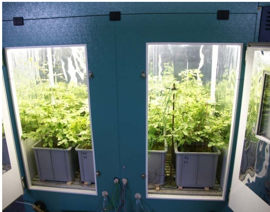
Fig. 6 - Frontal view of a phytotron with their eight containers. In two container six European beech saplings were subjected for a period of two years to 380 \mu\text{l l}^{-1} \text{h} and 680 \mu\text{l l}^{-1} \text{h} \text{CO}_2 fumigation respectively. Source: Fleischman et al. unpublished
