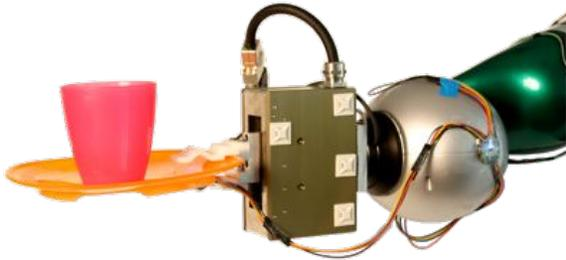
Fig. 12. Module mounted on gripper for orientation control
