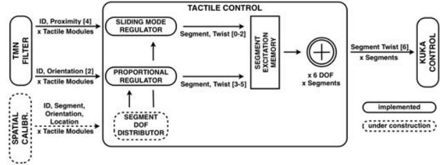
Fig. 7. Schematic overview of the Tactile Controller
