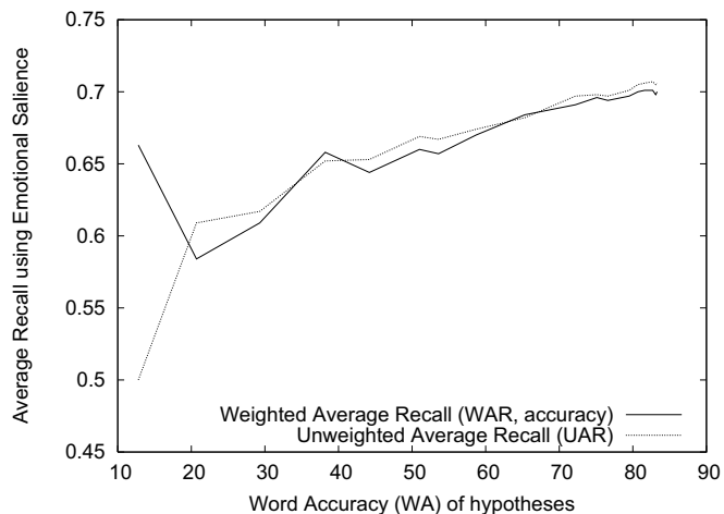
Figure 1: Recall versus word accuracy using 10-fold CV on the training data and an emotional saliency classifier trained on CMU/ T-Labs hypotheses.
