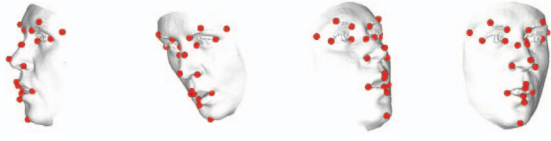
Fig. 1. Multiple views of one 3D facial surface. The facial feature points are manually labeled to build up a 3D ASM. When the facial surface is turned aside some facial feature points are occluded.
