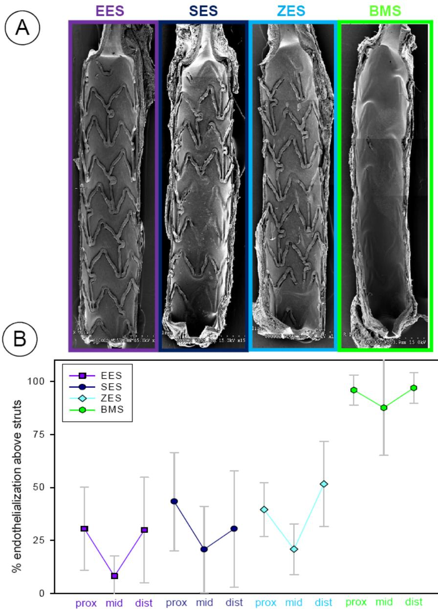
A. Low-power view of the entire luminal surface of each stent visualized per SEM. While the BMS shows almost complete tissue coverage of the strut surface, the DES constructs show uncovered and clearly visible stent struts, with only the very proximal and distal regions being buried under a tissue layer.
