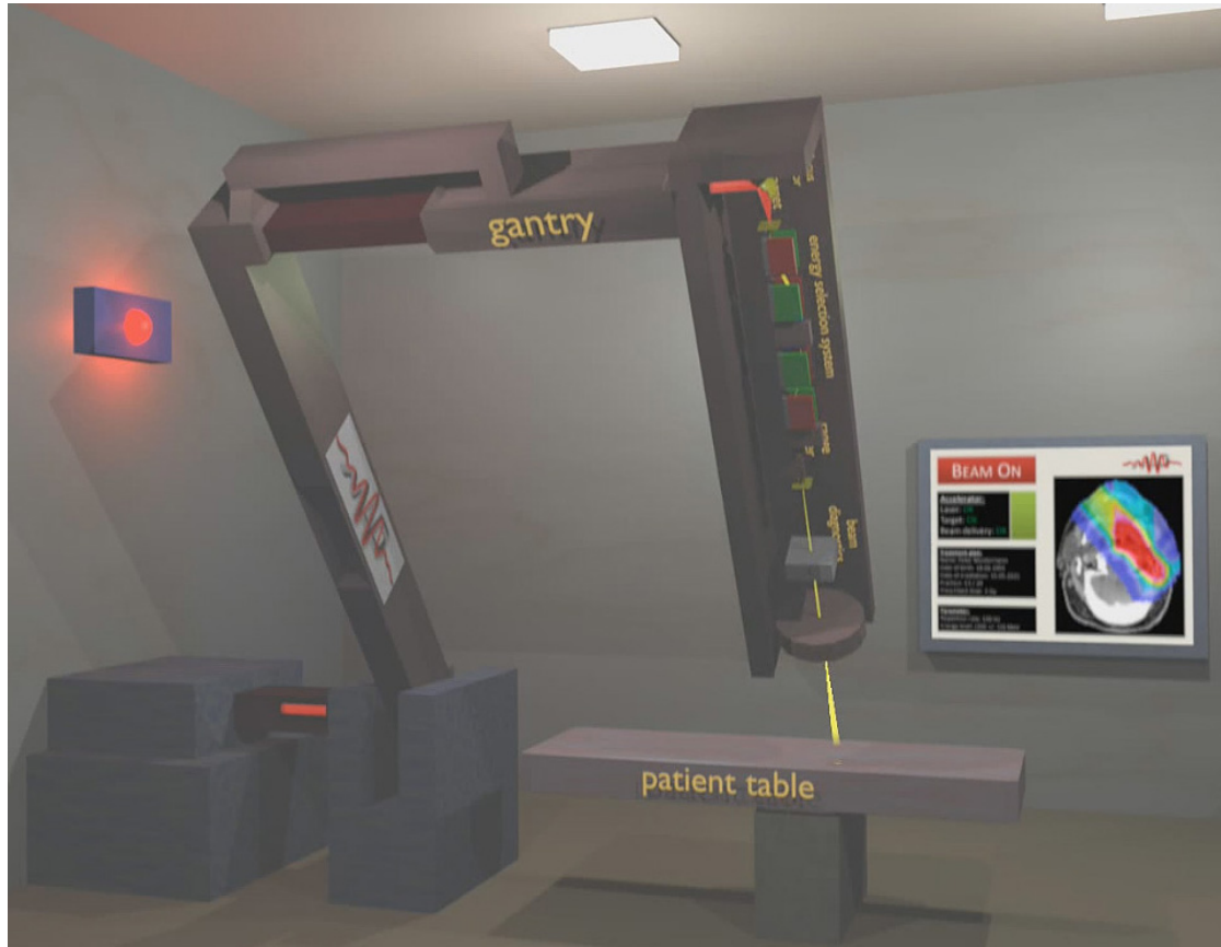
Figure 3.10: Rendering of a possible treatment room with a movable gantry for laser accelerated particle therapy. This screenshot is taken from a video prepared by the author that can be found at www.youtube.com/watch?v=0Gj2ht37TW0 . It shows the laser beam (red) coming from the bottom left which is guided through the gantry to the treatment head (open last part of the gantry displaying the elements of the beam delivery system). The particle beam (yellow) leaves the treatment head to irradiate a patient that would be positioned on the patient table.
