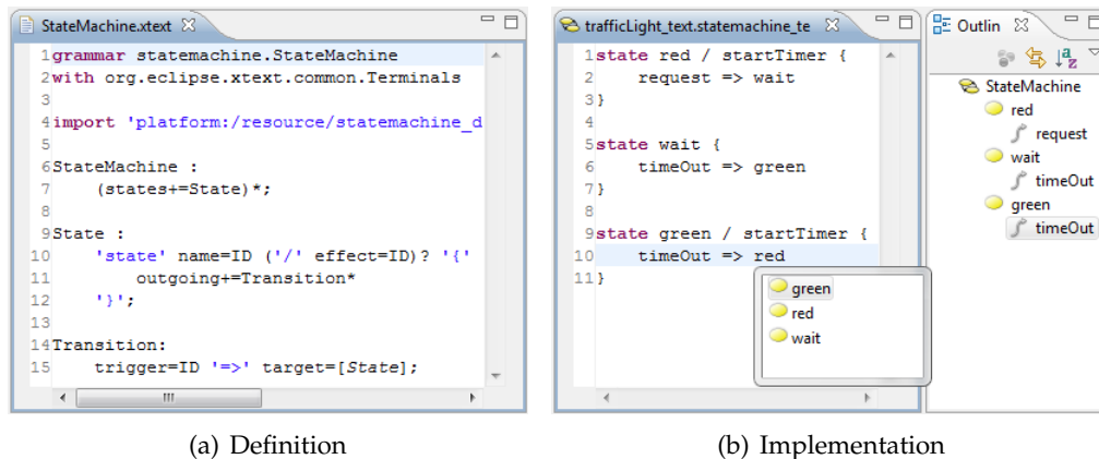
Figure 2.13: Textual concrete syntax in EMF
