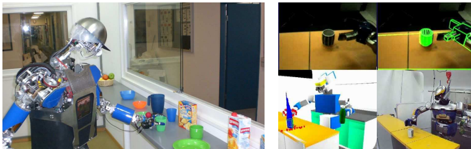
(a) Grasp execution with the humanoid robot ARMAR-IIIa using the developed object recognition and pose estimation system [4]
