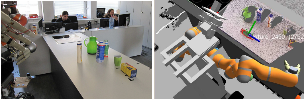
(a) A setup for the pick and place which is well segmentable. task. (b) A view of the verification step in Rviz, an object at a new position. task.
