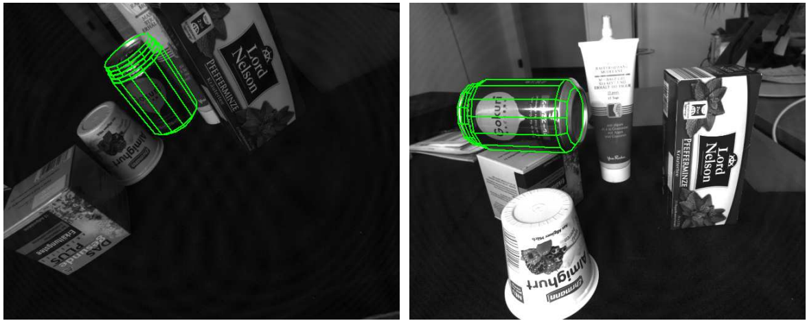
Figure 8.10.: Two objects matched based on descriptor points in cluttered scenes.
