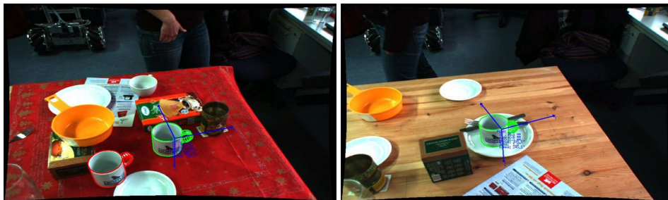
Figure 8.4.: Successful fitting object models in cluttered scenes. Several mugs are matched here.
