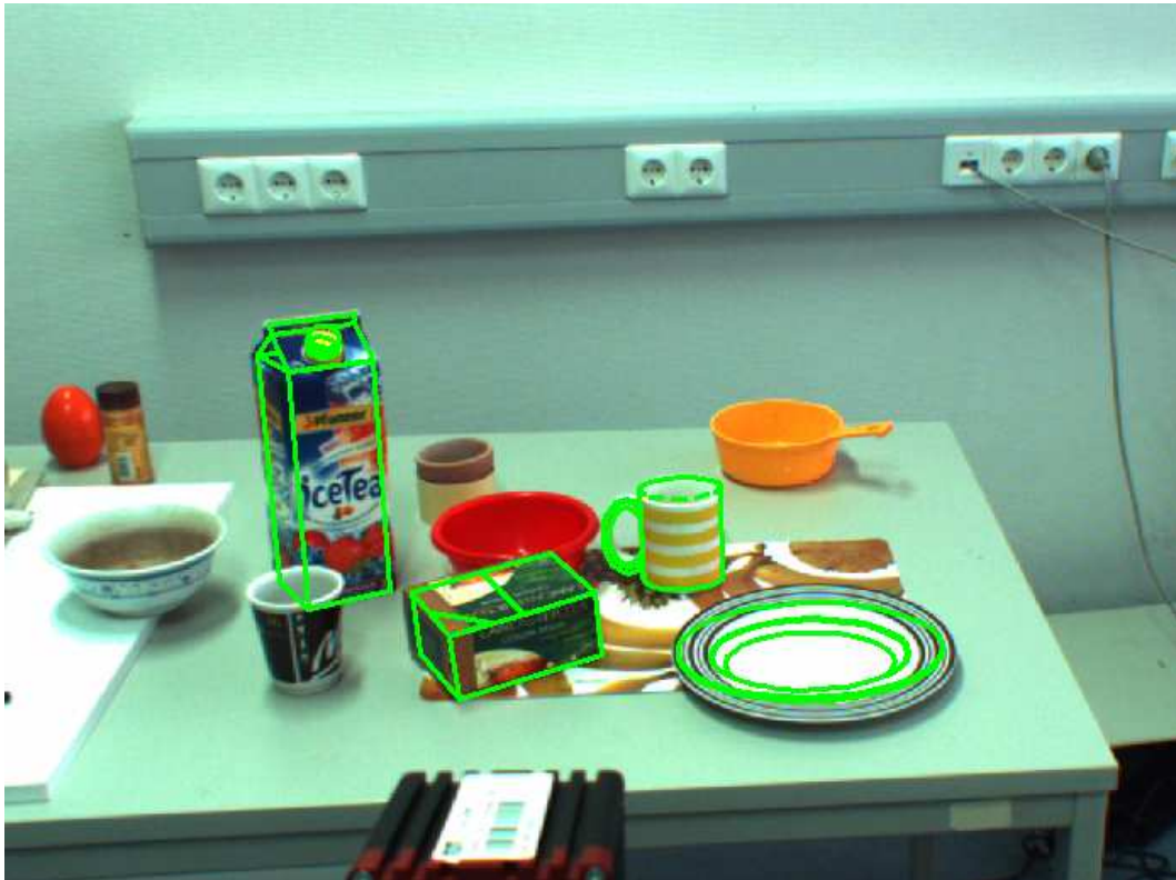
Figure 5.3.: Four different objects matched in a cluttered table setting. The projection of the matched CAD models is displayed in green.
