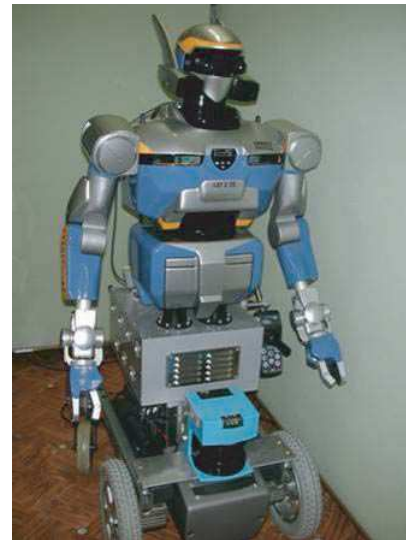
(b) The HRP-2W, the wheeled version of the HRP-2 with its sensor set [51].
