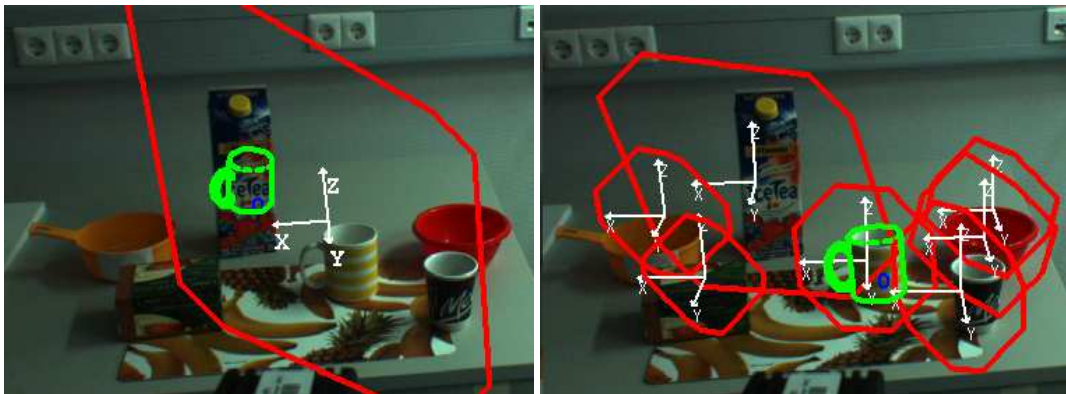
Figure 8.6.: An example of a single model search in a cluttered scene, using the entire search space (left), and using several regions of interest from the 3D processing module (right). Notice that the multiple RoI approach is robust against false positives, while in the full search space, the model of the mug is matched incorrectly.
