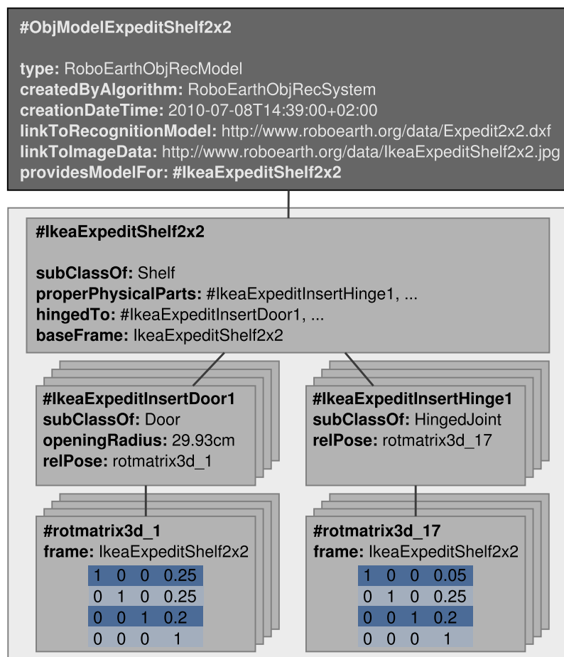
Figure 3.3 Description of an object recognition model (upper block) and the detection of an object using that model (lower blocks).
