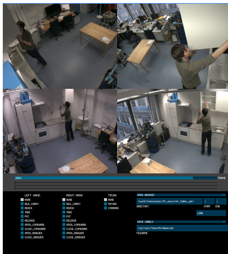
Figure 5.8 Screenshot of the labeling tool developed for annotating the human motions in the TUM Kitchen Data Set.
