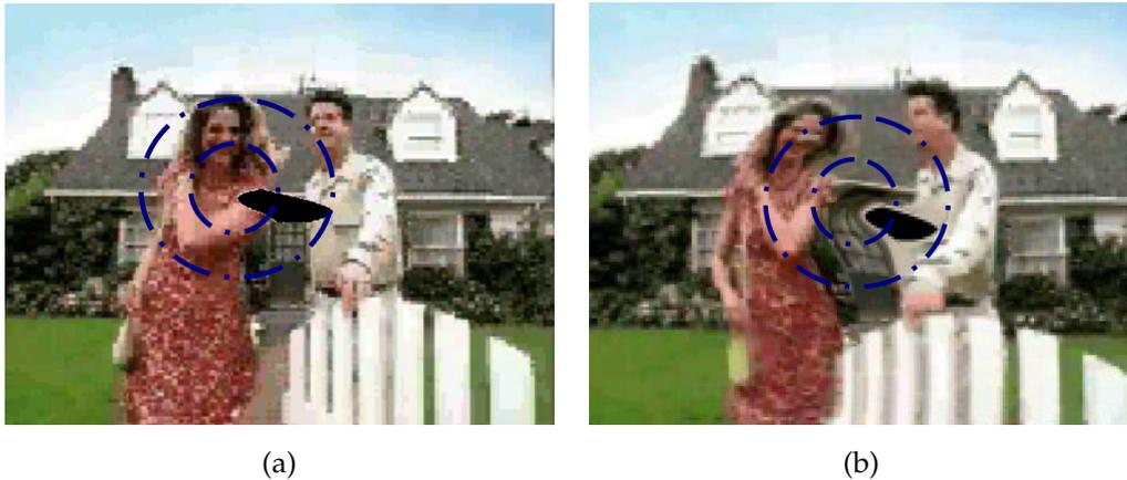
Figure 1.8.: ATDV system for patients with central vision loss [36]: (a) Original scene view, and (b) Scene view deformed by the ATDV system.
