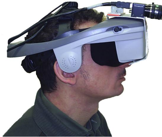
Figure 3.3.: Head-mounted magnification system for AMD patients.
