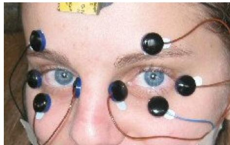
Figure A.2.: Electro-oculography: Skin electrodes placed around the eyes to collect electrical potential variations. (*Image source: [www.metrovision.fr](http://www.metrovision.fr)*).
