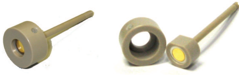
Figure 5.2: Photo of the proton source assembled (left) and disassembled (right). The gold-colored disc is the americium alpha source. The cylindrical cap holds the mylar foil.
