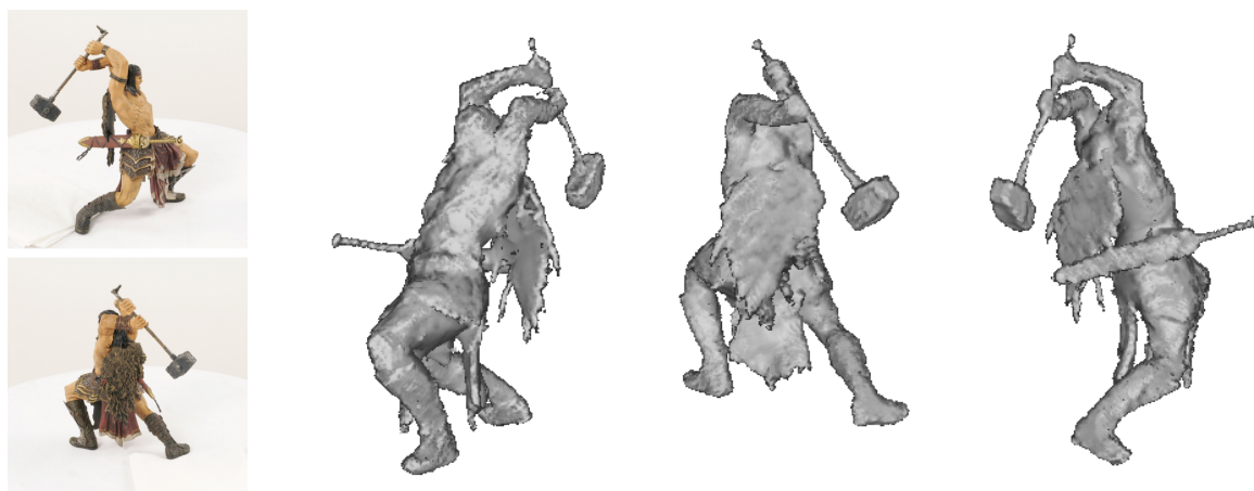
Fig. 4.8: Warrior sequence. 2 out of 24 input images of resolution 1600 \times 1600 and multiple views of the reconstructed surface. Note that thin structures (for example the handle of the hammer) as well as concavities (for example at the chest) are reconstructed accurately.
