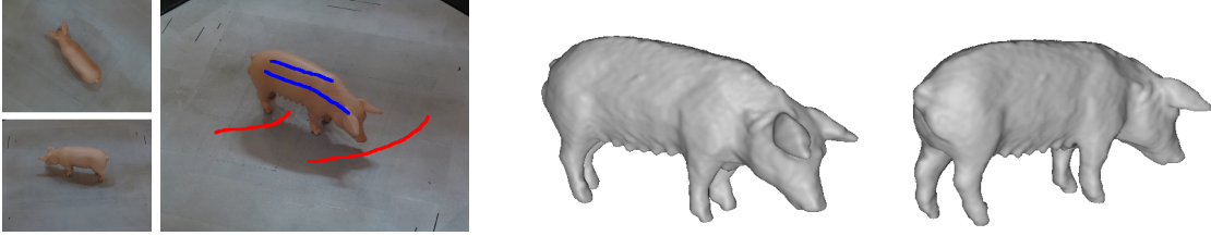
Fig. 2.1: Surprisingly accurate reconstructions can be obtained from a few scribbles marking foreground and background in only one of the input images of a sequence. Such an approach is in contrast to classical shape-from-silhouette methods, where all silhouettes are extracted explicitly in advance, which entails considerable interactive efforts.
