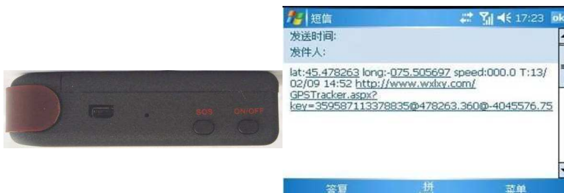
Figure 6.16 Location position that can be sent via a wireless tracker with an SOS button
