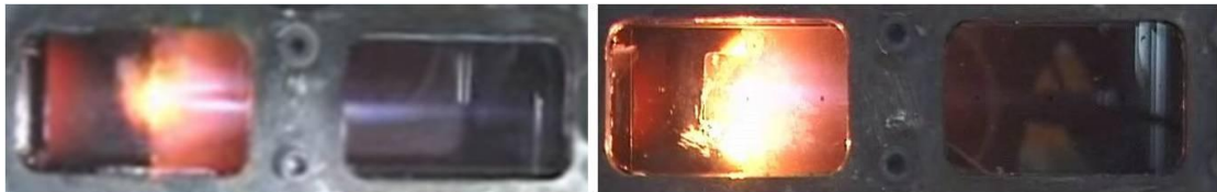
Figure 4.21 Near stoichiometric pilot flames stabilized with Strut 1 (left) and with Strut 3 (right).
