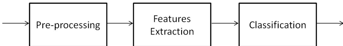
**FIGURE 2.2** Generic flow of a face recognition system
