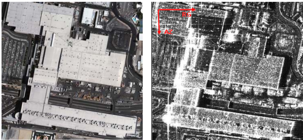
Fig. 7: Optical image of Las Vegas Convention Center (left) and corresponding mean TerraSAR-X intensity image (right).
