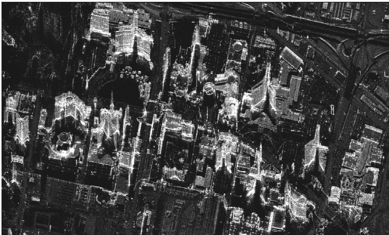
Figure 1. TerraSAR-X mean intensity map from 30 images of a high rise urban area over downtown Las Vegas with a spatial resolution of 1.1 \text{ m} \times 0.6 \text{ m} in azimuth and range.
