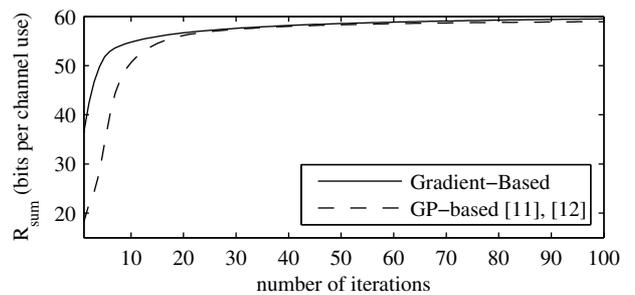
Fig. 2. Convergence of the GP-based and the Gradient-based Algorithm for  $P = 20$  dB.
