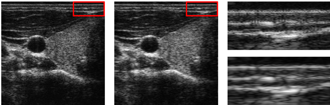
Figure 3.6: Log-compressed envelopes from 1D ASF (left) and 2D ASF (middle). Magnification of red region (top right: 1D AS, bottom right: 2D AS).
