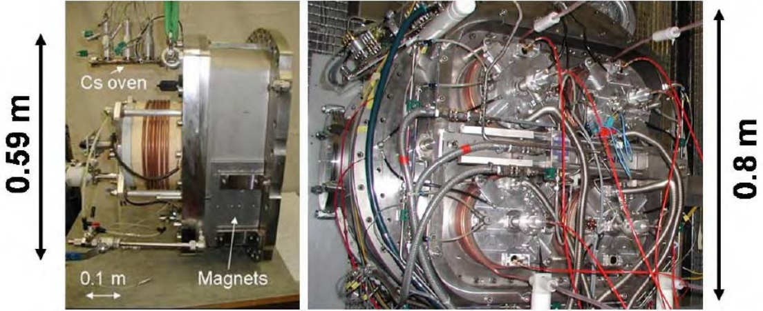
Figure 3.9: Ion source of MANITU (left), with a single driver, and of RADI (right), with four (2x2) RF-drivers. The RADI source is approximately half the size of the ITER source (with 2 \times 4 drivers).
