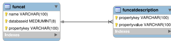
Figure 1.21: Example of two tables and their relation within the ChlamydiaeDB The figure shows two tables, the table "funcat" and the table "funcatdescription". "funcat" contains information which proteins are annotated with which Functional Catalogue (FunCat) categories. name is the proteinname (e.g. Gl:10957571), databaseid is an internal databaseid referencing another table not shown here (e.g. 711 for Chlamydia muridarum Nigg) and propertykey is a FunCat category (e.g. 11.02.03). The description for the FunCat categories is stored in the table "funcatdescription". propertykey is a FunCat category (e.g. 11.02.03) and propertyvalue is the associated FunCat description (e.g. mRNA synthesis). The propertykey of "funcat" and the propertykey of "funcatdescription" reference each other and define a relation: using the propertykey of "funcat" the description can be retrieved using the same propertykey in table "funcatdescription". This separate storage of FunCat categories and FunCat descriptions makes it possible that the FunCat description has not to be stored for each of the annotated proteins in the table "funcat". In order to retrieve the complete information for a protein a join between the two tables has to be done using the common column "propertykey".
