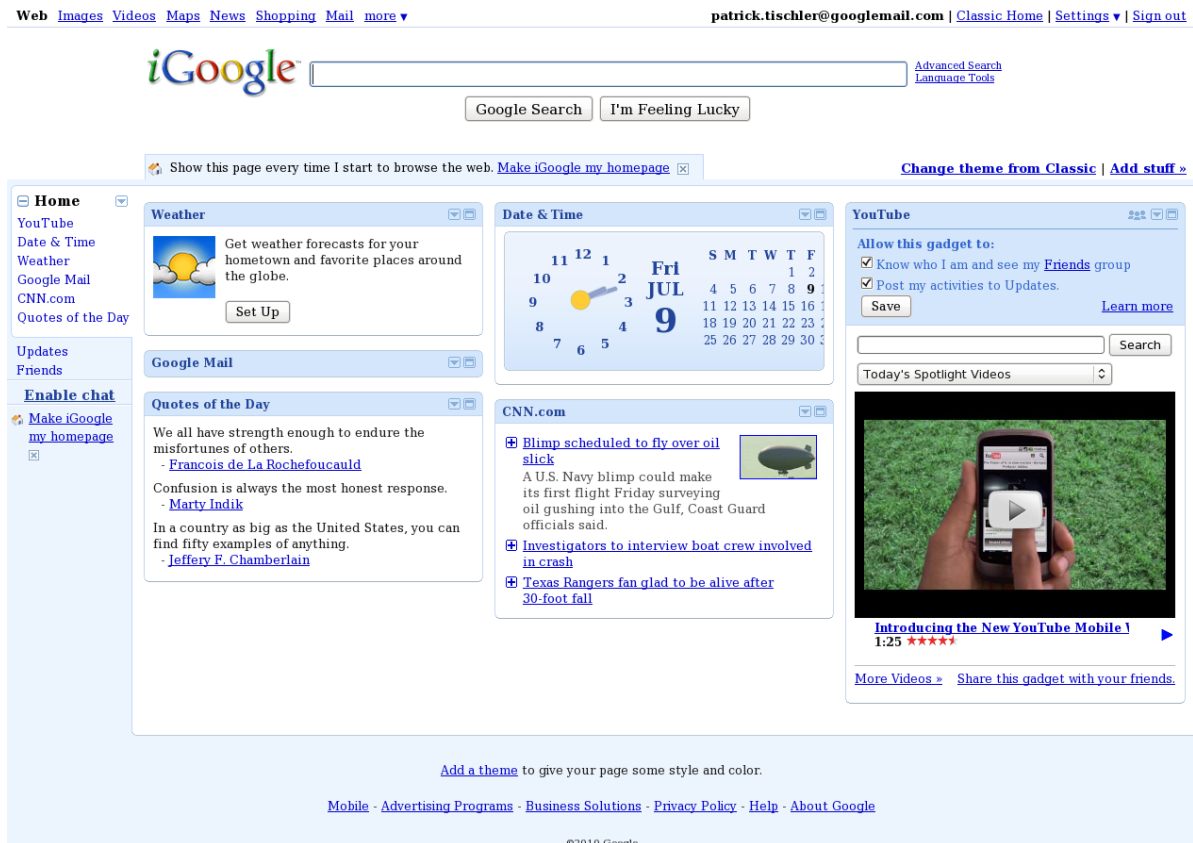
Figure 1.22: The iGoogle portal page There are different programs visible. These programs (portlets) are Weather, Date and Time, Youtube, CNN.com, Google Mail, Quotes of the Day. The iGoogle portal provides a consistent look and integrates the different programs into a single page.
