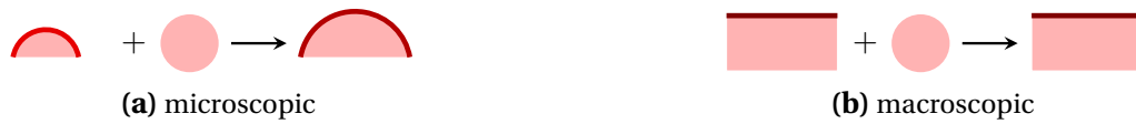
Figure 4.5.: The integration of a new particle into the growing solid has an impact on the surface energy in a microscopic but not in a macroscopic configuration.
