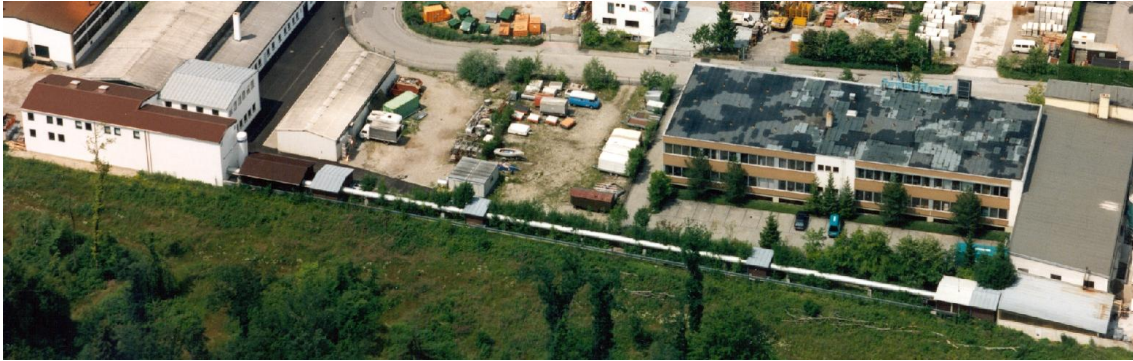
Figure 4.5: Aerial view of the PANTER X-ray test facility in Neuried (to the south of Munich). The small shed on the right contains several X-ray sources. The building on the left is the main building, which houses the test chamber and the control room, among others. In between the two buildings, the 120 m long, 1 m diameter vacuum tube with the two auxiliary pumping stations are visible.
