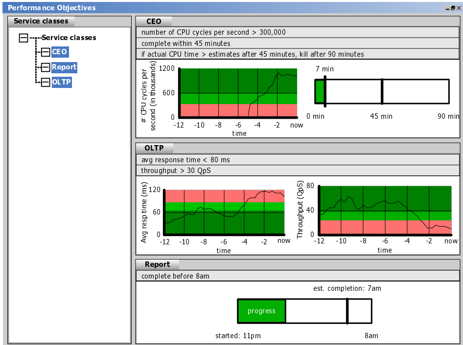
Figure 5.17.: Performance objective screen after problem injection shows the OLTP service class not meeting objectives.
