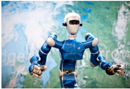
Figure 6.14: DLR humanoid robot Justin looks quite human-like and friendly when the arms are in a configuration that appears comfortable for a human. Justin can move in a very human-like manner, but it can also perform movements that look very awkward for a human observer.
