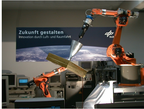
Figure 6.9: The ESS demonstrator simulates the approach and docking of a robot arm to a tumbling satellite. A Kuka industrial robot approaches a satellite and captures it using the capture tool developed at the DLR.
