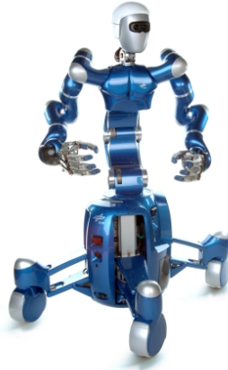
Figure 6.1: The DLR mobile humanoid robot Rollin' Justin . Two DLR LWR arms are attached to an upper body. The omni-directional mobile base has a variable foot print.
