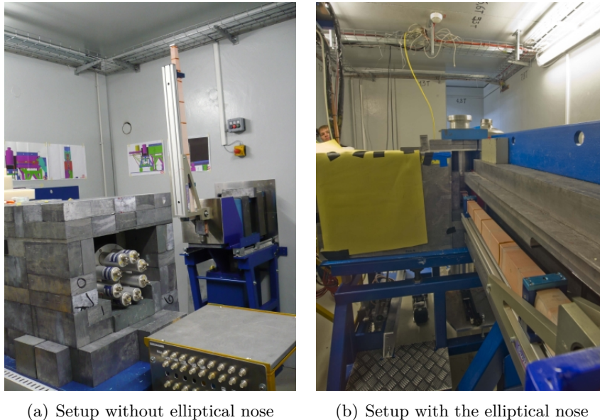
Figure 3.3: The two different setup available at the PGAA instrument. Without 3.3(a) and with 3.3(b) elliptical nose. 1
