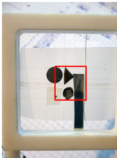
Figure 5.7: Sample used for the 2D-PGAA imaging with different materials. The scanned area is highlighted.
