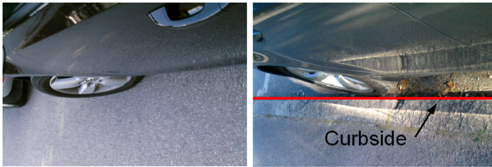
Figure 3.16: Left: Parking on the ground plane. Right: Parking close to the sidewalk. The curbside of the sidewalk may be used to identify parking situations that have an offset \Delta between the ground plane and the car ground plane.
