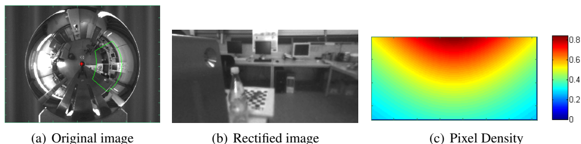
Figure 2.40: Original image with highlighted region of interest (a). Rectified image using plane projection (b) and its characteristic of the pixel density (c).
