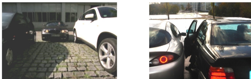
Figure 1.1: Cars parked in tight parking lots. The car doors cannot be opened wide enough to provide optimal space for comfortable ingress/ egress.
