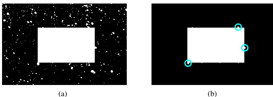
Figure 3.25: Simulated foreground object and extracted snowflakes (a). Removed snowflakes using median-filtering and remaining disturbances at the boundary of a detected object (b).
