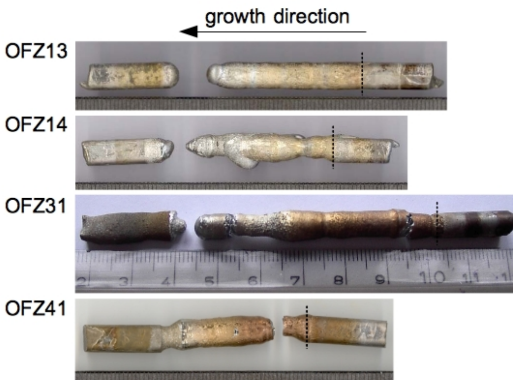
Figure 6.1: The four \text{Fe}_2\text{TiSn} crystals grown in the course of this thesis. The first crystals OFZ13 and OFZ14 were grown with a growth rate of 10 mm/h and 5 mm/h, respectively, resulting in a poly-crystalline structure. Crystals OFZ31 and OFZ41 were grown with a reduced growth rate of 0.7-1 mm/h, resulting in large single-crystalline grains. The dashed lines mark the beginning of the growth with the growth direction to the left. The formation of oxides causes the weak yellow staining of the crystals.
