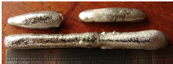
Figure 7.3: \text{NbFe}_2 starting rods for crystal OFZ12 prepared by William Duncan in a horizontal furnace with RF induction heating.
