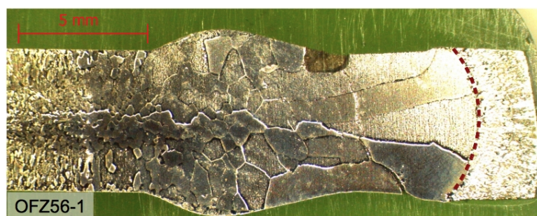
Figure 5.5: Longitudinal cut through crystal OFZ56 at the beginning of crystal growth. The growth direction is from left to right. The grain selection process abruptly stops at a well-shaped convex growth interface marked by the dashed red line. EDX-analysis revealed an excess of manganese to the right hand side of the interface.
