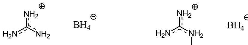
**Scheme 34: molecular structures of guanidinium and methylguanidinium borohydrid.**
